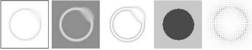
Figure 10.16: Diffused region force on weak edge. From left: the edge map, the stopping function g(\cdot) of edge map, the magnitude of its gradient \nabla g(\cdot) , the region segmentation map, and the vector map of the diffused region force \tilde{R} .
