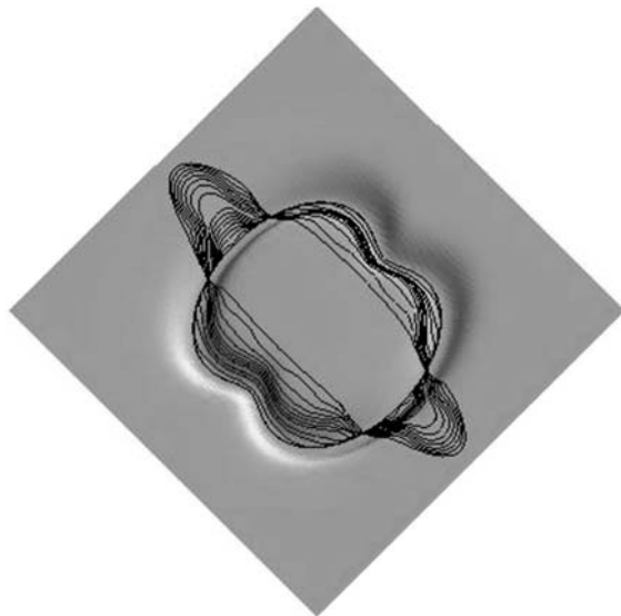
Figure 11.6: An initial ellipse driven by the vector field -\nabla g(|\nabla I^0(x)|) down to the valley to find the edge in the image I^0 (color slide).
