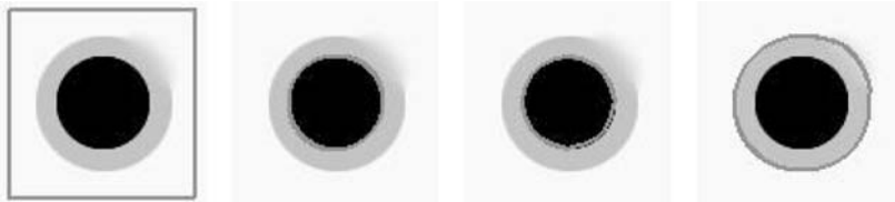
Figure 10.17: Strong neighboring edge leakage. From left: initial snake, geodesic snake steps through weak edge in top right of outer boundary, GGVF is attracted by the stronger inner edge, and RAGS snake converges properly using extra region force.
