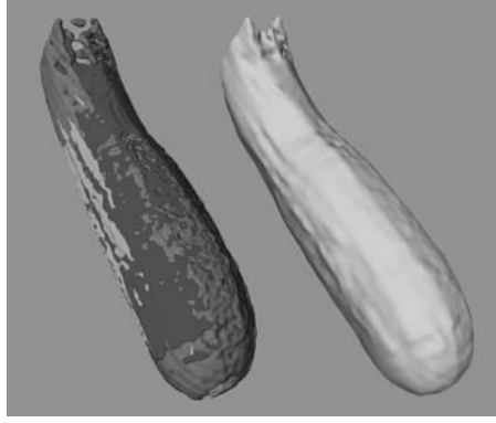
Figure 8.10: Three low-resolution MR scans of a zucchini that have been individually colored and overlaid to demonstrate their imperfect alignment. The level set model on the right is derived from the three low-resolution scans.
